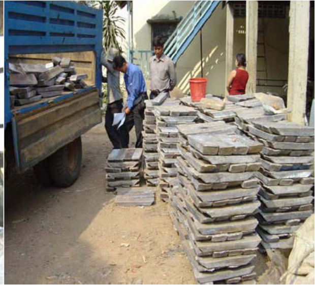
Picture 20: Ingots from the lead melter
