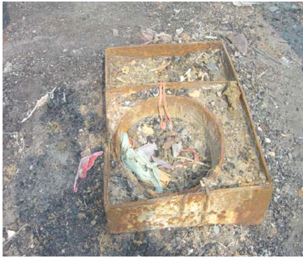
Picture 26: Crude smelting furnace
