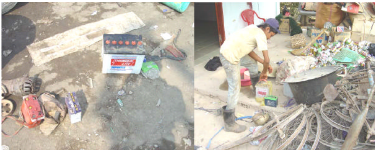
Picture 17: Battery acid drained into the ground at the collection sites
