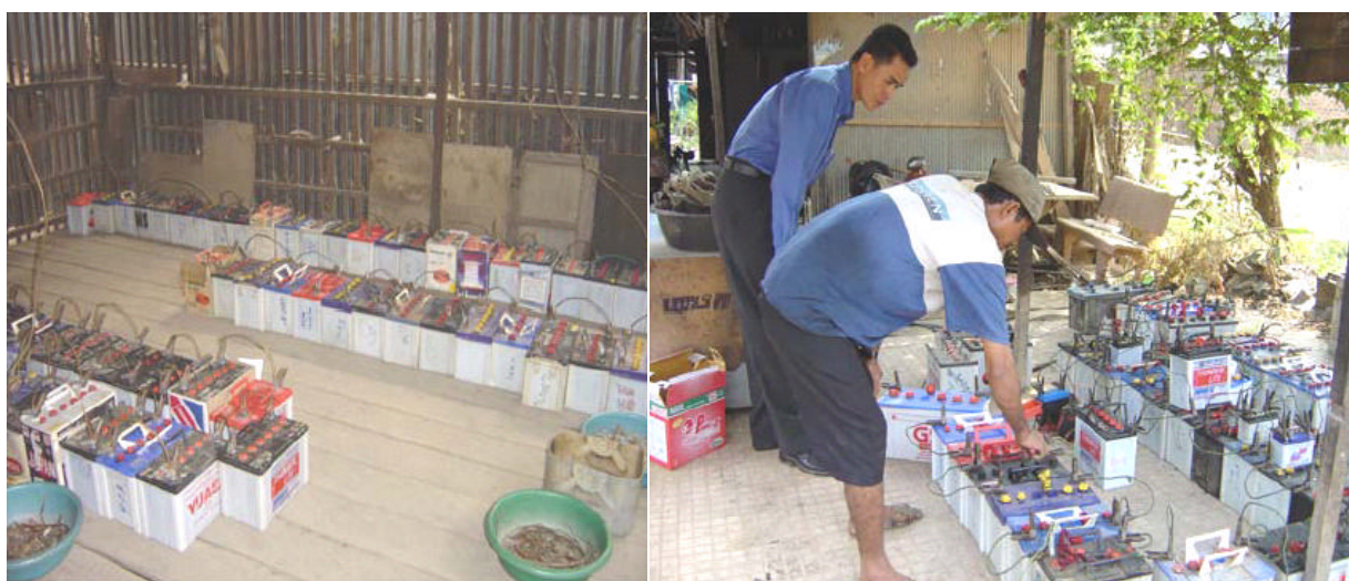
Picture 7: Batteries are charged in series
