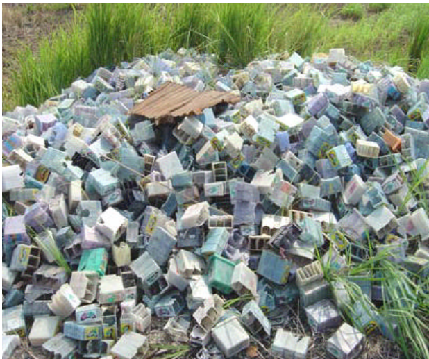
Picture 24: Battery cases after breaking
