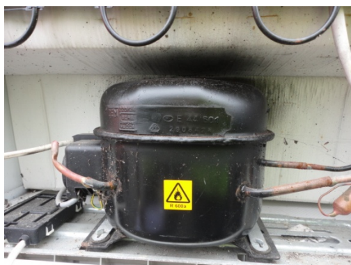
Faked stickers on compressors of refrigerator
