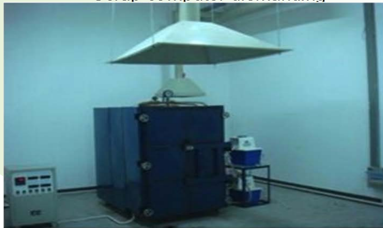
Furnace for LCD and thermal shock treatment of PCBs
