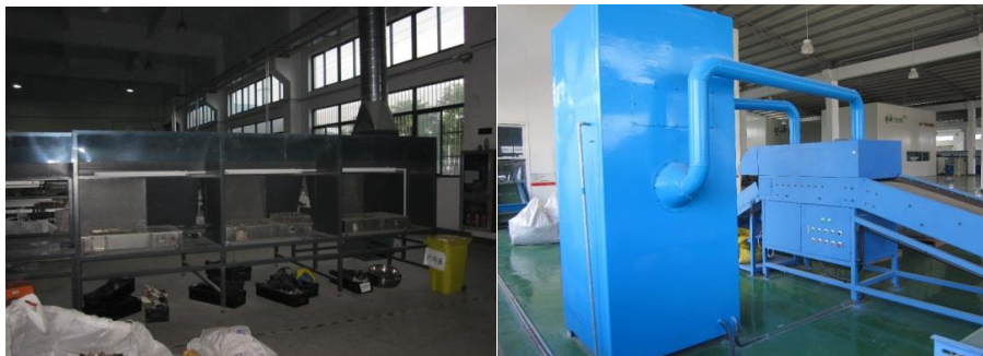
Fig. 4-13 Solder heating device and physical cutting device
