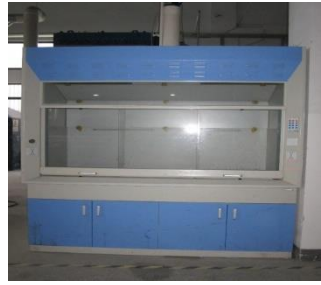
Fig. 4-5 Sealed vacuum LCD dismantling platform
