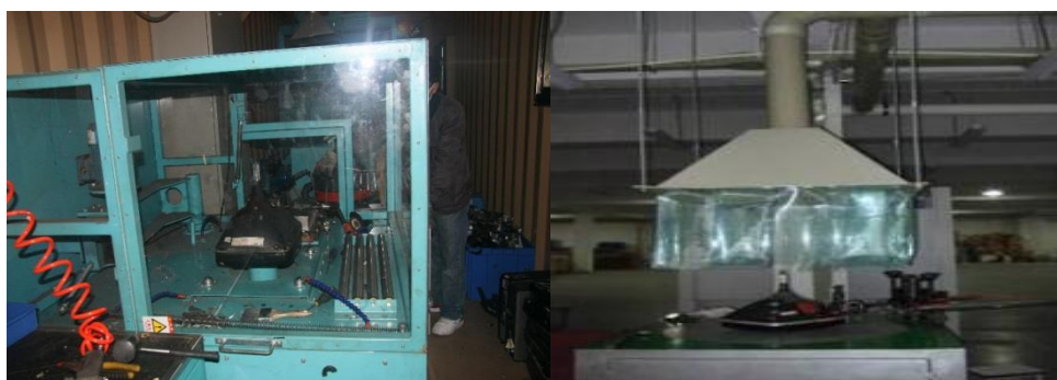
Fig. 4-11 Separating equipment for CRT glass using heating wire method
