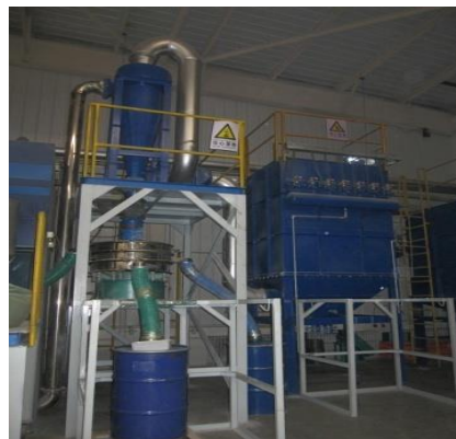
Fig. 4-9 Refrigerator crush and separation equipment
