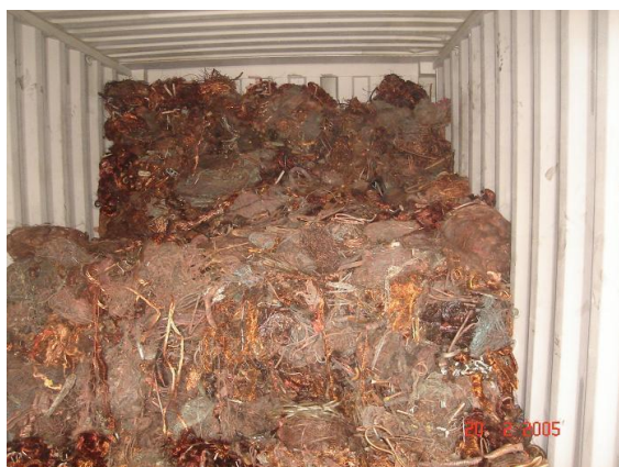
Sorted and processed copper wire – stripped in a simple cable stripper - in a shipping container for export.
