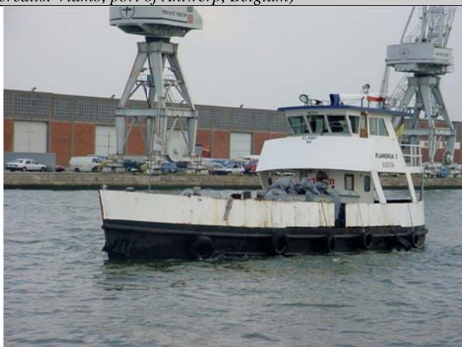
Example of a barge collecting solid wastes only (Photo credits: Vlamo, port of Antwerp, Belgium)
