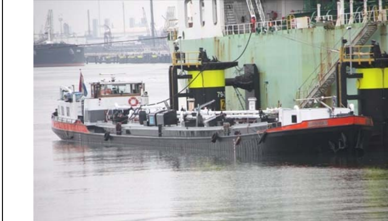
Example of a barge collecting oily wastes (Photo credits: Martens Vlissingen, NL)
