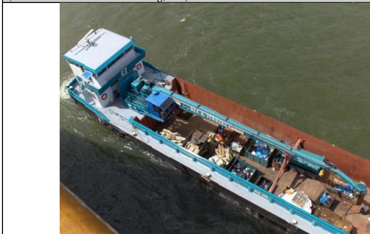
Example of a barge used for collecting garbage in the port of Rotterdam (Photo credits: Bek & Verburg, NL)
