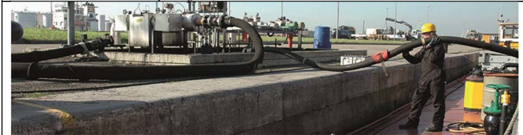
Example of a collection barge delivering oily waste to a fixed port reception facility for further processing (Photo credits: MAC2 Antwerp, Belgium)
