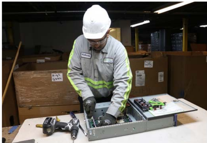
Figure 2: Manual dismantling of e-Waste (Source: http://www.theepochtimes.com/ )
